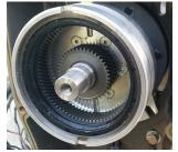
transmission and Sun Gear. Set the rotor on a shop towel with the internal gears facing upward.
