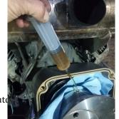
about 1 inch. Carefully empty the 1.25 oz of 10W30 oil into the transmission. Reinstall the drain plug and wipe up any oil drips.
