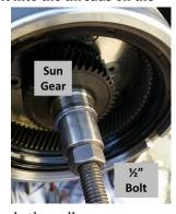
washers. Steady the puller arms around the washer with one hand while sliding the hammer to pull the gear off
